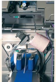
Infeed and outfeed conveyor Pneumatic grippers Vertical side belts Product sensors
