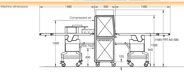
The FRT-A machine offers virtually hands free operation. With amazing speed and consistency, this fully automatic machine is able to transform cuts of meat into attractive case-ready products. Its ease of operation and versatility allows adjustable spacing, number of ties,
