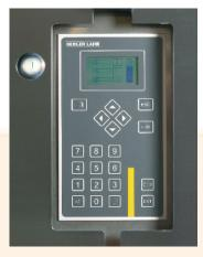
Number of strings Desired twine spacing Belt speed Self diagnostic error messages Two level resettable cycle counter
